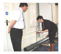
rig to demonstrate how to measure air flows and performance correctly, and how easy it is to get false readings. We were able to have hands on experience of doing this.
